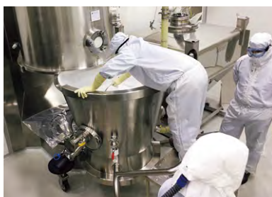
Local staff is taking out granulated active ingredients at the new plant Unit 7.
