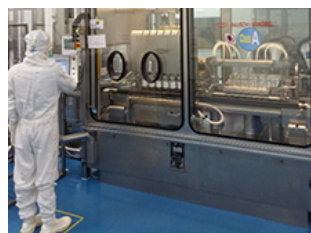
Filling process for sulbacillin (PT. Meiji Indonesia Pharmaceutical Industries, Bangil Plant)
