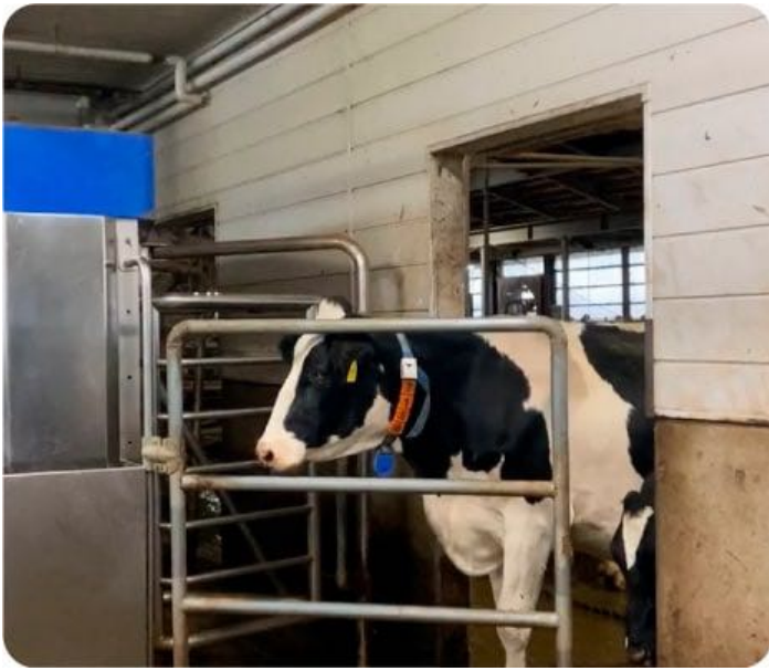
A cow entering the milking robot. The machine reads an information tag attached to the cow's neck and identifies the individual information.
