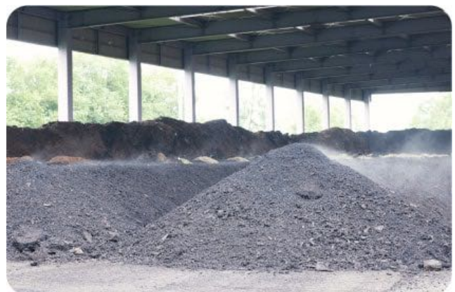
During fermentation, the temperature rises to 70-80°C.
